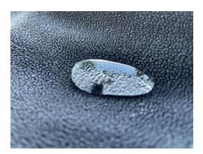
The same properties that make PFAS bioaccumulative and difficult to remediate is the strong fluorine bond demonstrated here showing water beading up off a water repellant treated textile.
