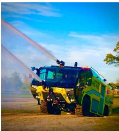
An ARFF - Aircraft Rescue & Firefighting - vehicle shown in action. Photo by William Greenwood
